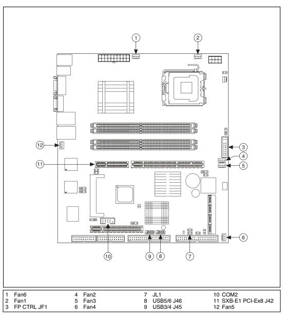
Figure B-10 shows the locations of other connectors on the NI 8352/8353.
